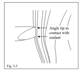
Align the adjustment tool to the edge of the door, with the angle edge positioned toward the inside of the door (Fig. 3-3).
